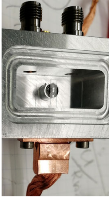
Figure 4.6: Photograph of one half of a rectangular waveguide cavity with two transmon qubits fabricated on one sapphire piece, separated by a distance of 2 mm along the z-axis. The cavity is machined with an empty cylinder in the middle of the back wall to insert a magnetic hose. On the bottom of the cavity, a copper clamp is used to hold and thermalize the sapphire. On top of the cavity two holes are machined for the insertion of two pins, that act as antennas. SMA connectors are used to hold the pins and couple the cavity with the external environment. More details in chapter 5.
