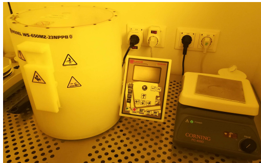
Figure 20: Picture of the spincoater and the hotplate which are used for qubit fabrication.
