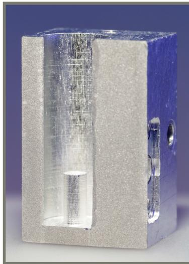
**Figure 4.5:** Picture of the etched high purity aluminum coaxial  $\lambda/4$  resonator. After the measurements were finished, a vertical cut was carried out to make the inside of the cavity visible.
